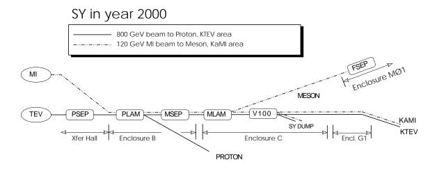
Figure 7.1. Schematic of the switch yard configuration allowing 120 GeV MI beams to be delivered to the meson area.
